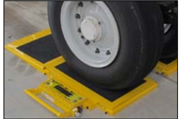
Aircraft weighing: dual wheel configuration with AC40-LP aircraft platform scales
